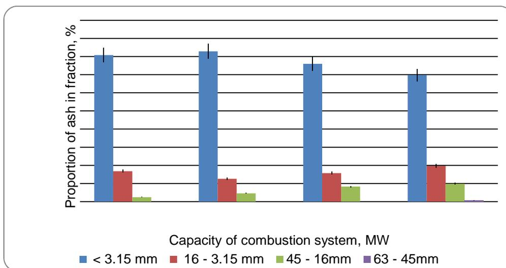
**Figure 2** Ash fractions depending on capacity of combustion system.
