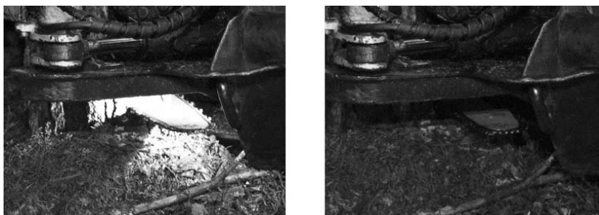
Figure1. The area around the stem base, with and without the additional lights in the harvester head. Pictures from the very first trial.
