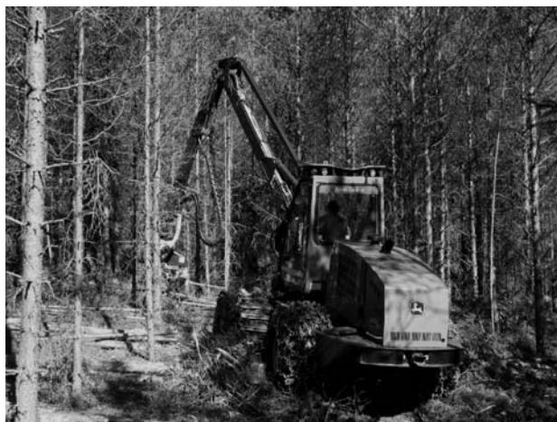
Figure 1. A harvester is processing small-sized thinning wood.
