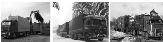
Figure 2. A biomass truck equipped with solid side panels and bottom (left), a standard chip truck and a standard timber truck (right).
