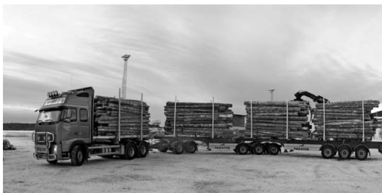
Figure 1. The studied vehicle, loaded with 65 tonnes at one of the terminals.
