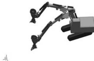
Figure 2. The two-armed excavator base machine model.
