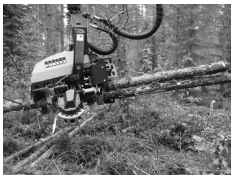
Figure 1. Multi-tree handling of pulpwood-dimensioned stems with the Ponsse Ergo 8w/H7 in the time study. Photo: Antti Perho.
