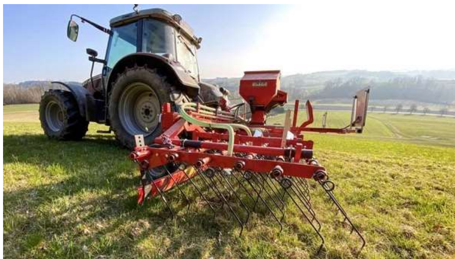
Figure 1. Einbock PNEUMATICSTAR seeder 2 .
