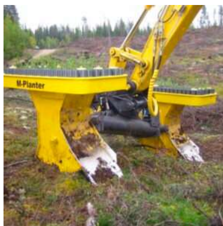
Figure 7. M planter M240 seedling machine 9 .
