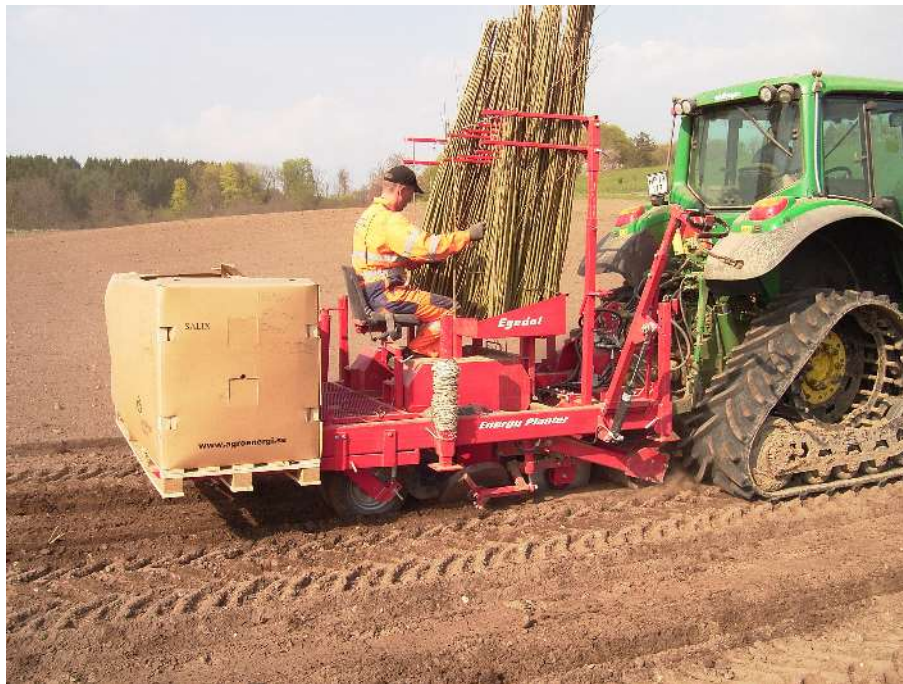
Figure 4. Two-row cuttings seedling machine 6 .
