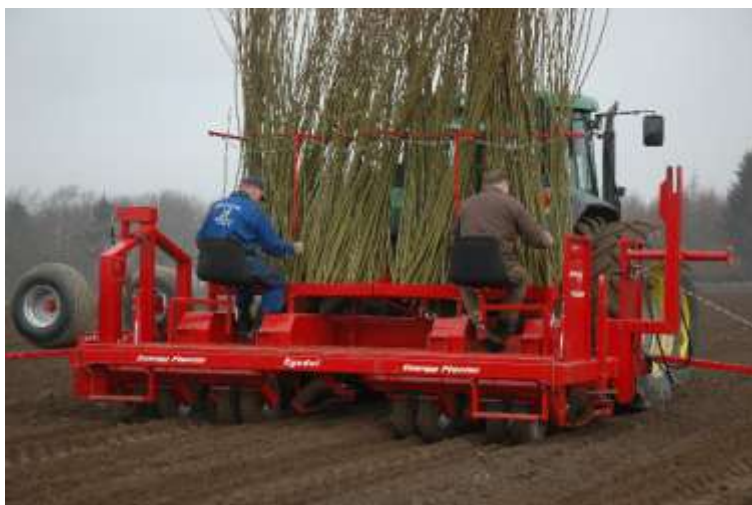
Figure 5. Four-row cuttings planter 7 .
