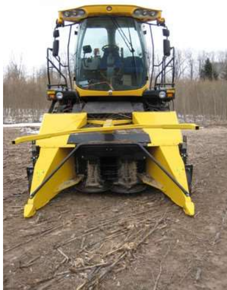
Figure 15. New Holland FR9090 with 130 FB working head. 18
