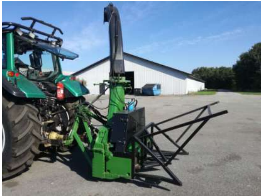
Figure 16. John Deere 8520T with JF Z200-HYDRO C2 working head. 19
