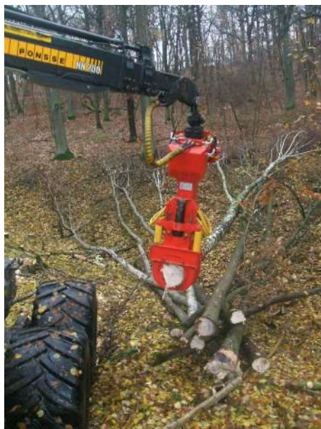
Figure 17. Naarva Grip 1600-40 working head 20 .
