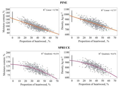
Figure 1. Wood moisture and density (freshly felled) changes depending on heartwood proportion.
