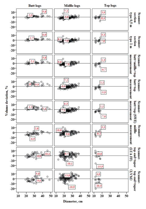
Figure 1. The difference of volume compared to scanner for pine assortments.
