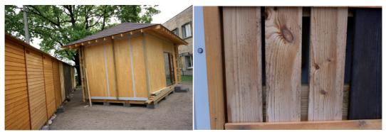
Figure 1. Open air study field for wood cladding surface finishing efficiency monitoring.
